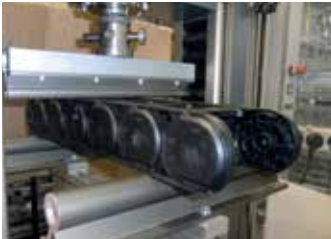
Strength test to determine maximum unsupported length
