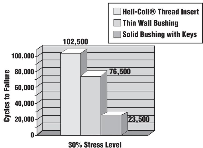
IN ANOTHER TYPICAL FATIGUE STUDY, the load per turn has been shown to be far better distributed with Heli-Coil® inserts than in plain tapped holes. The actual percent improvement of stress distribution is shown in the following graphs taken from the report on this study.\*
