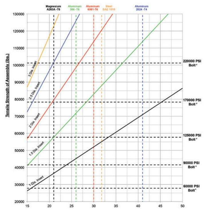
Shear Strength of Parent Material (ksi)
