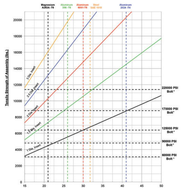
Shear Strength of Parent Material (ksi)
