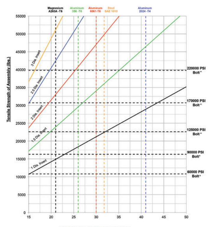
Shear Strength of Parent Material (ksi)
