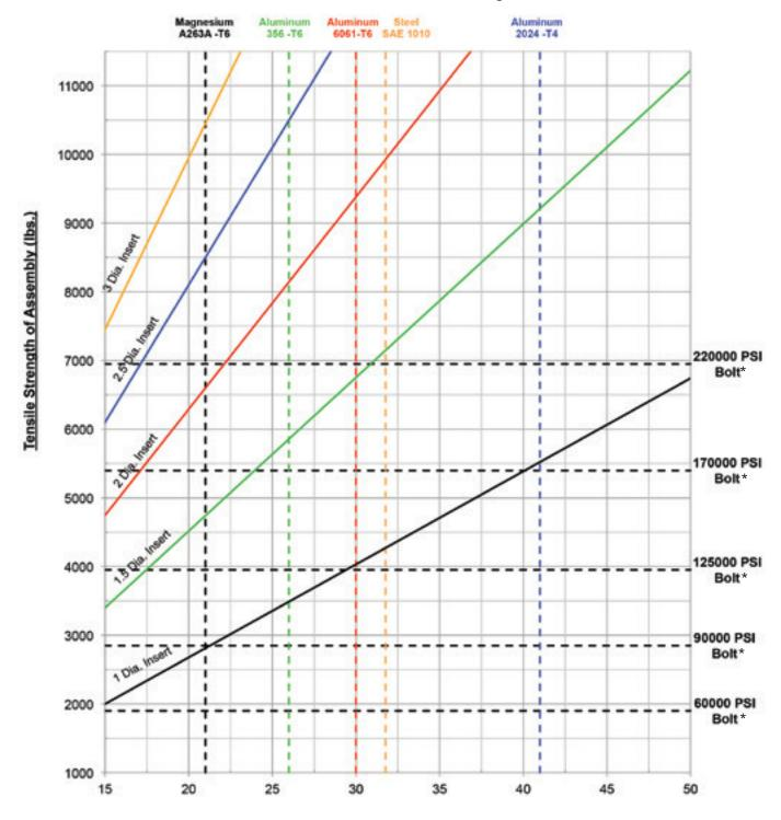
Shear Strength of Parent Material (ksi)
