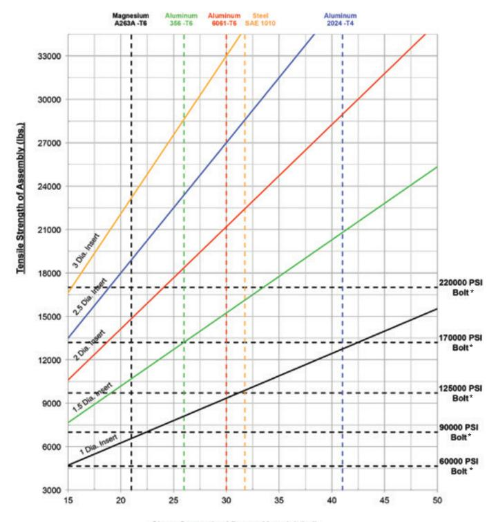
Shear Strength of Parent Material (ksi)
