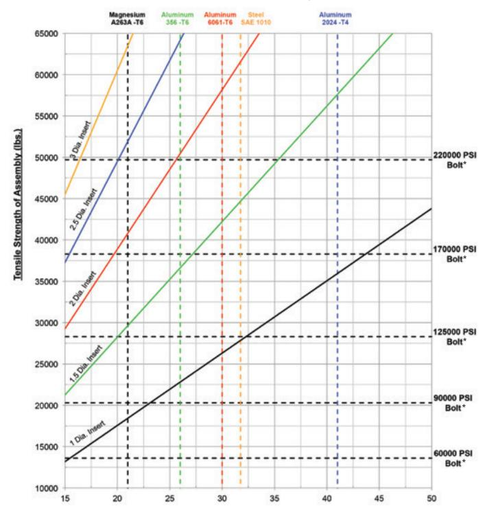
Shear Strength of Parent Material (ksi)
