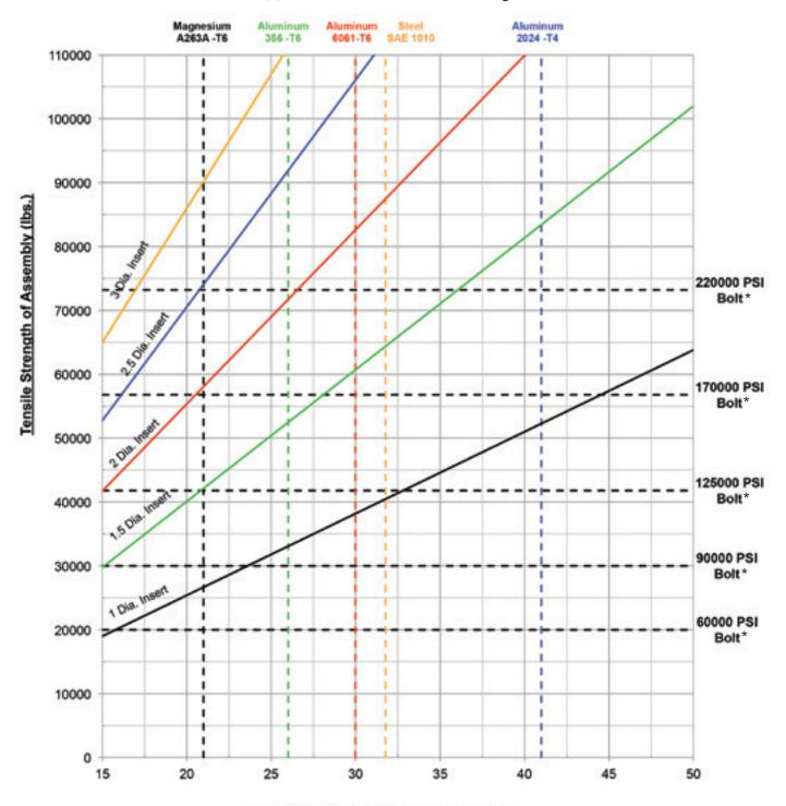
Shear Strength of Parent Material (ksi)
