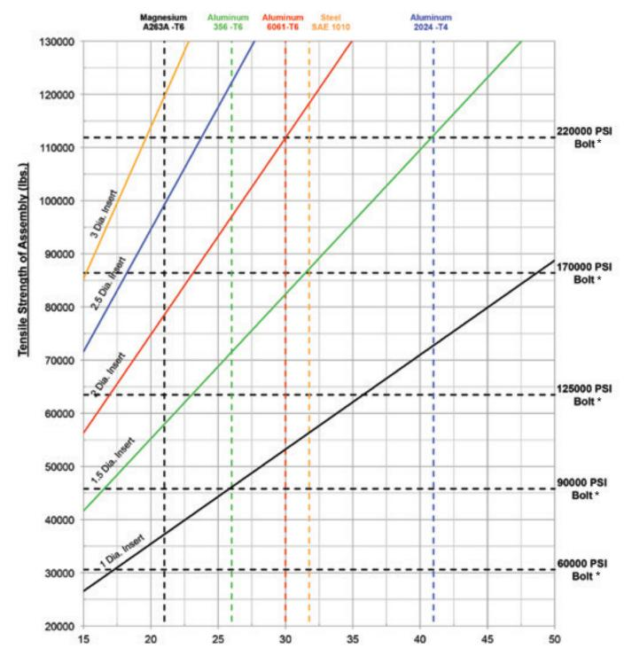
Shear Strength of Parent Material (ksi)
