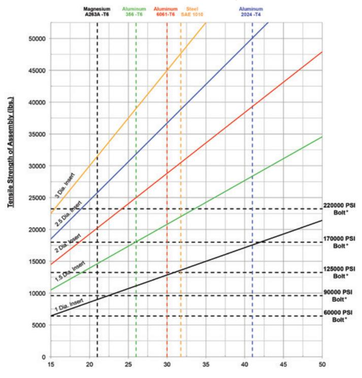
Shear Strength of Parent Material (ksi)
