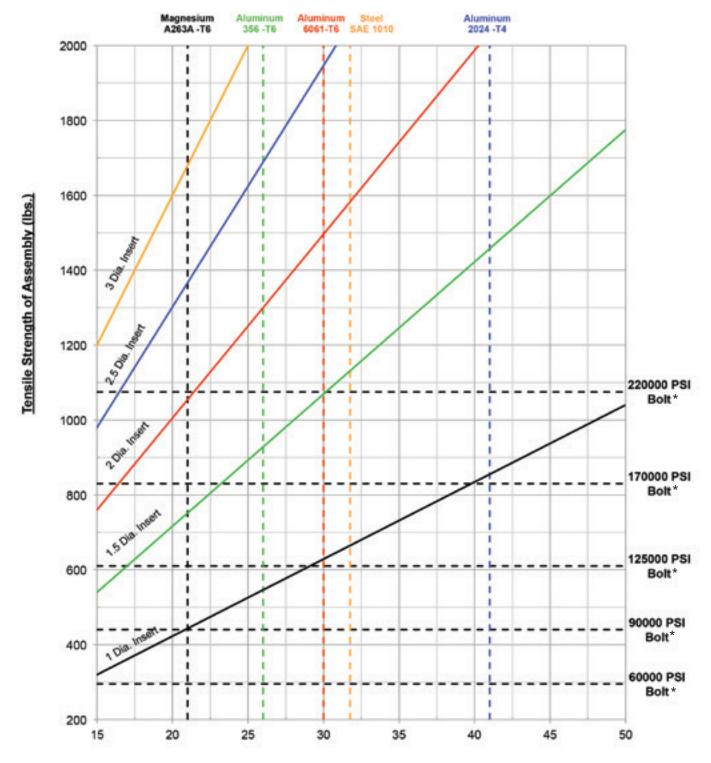
Shear Strength of Parent Material (ksi)
