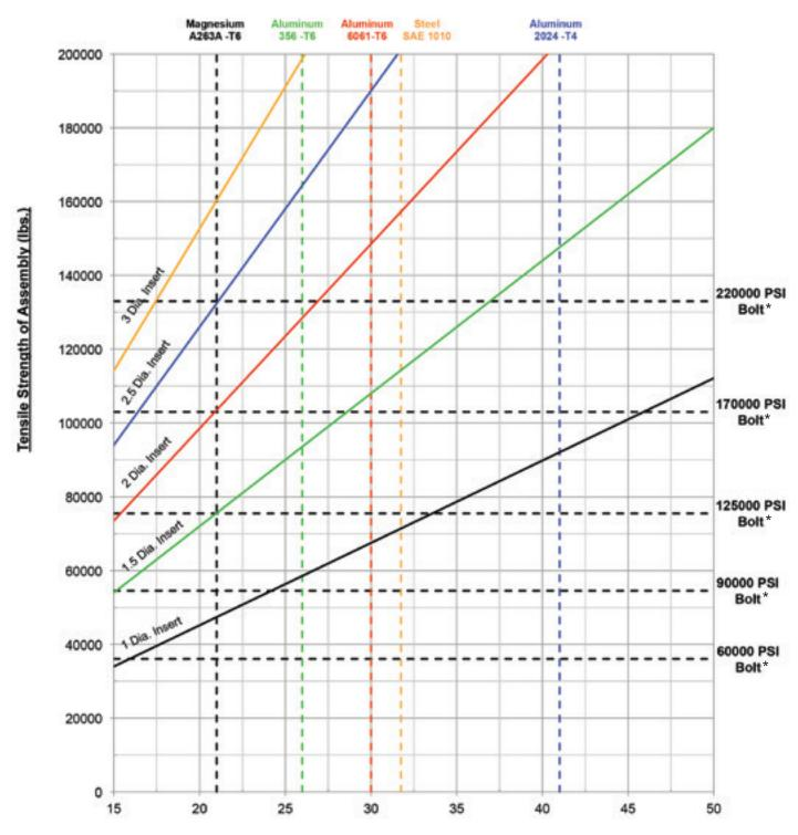
Shear Strength of Parent Material (ksi)
