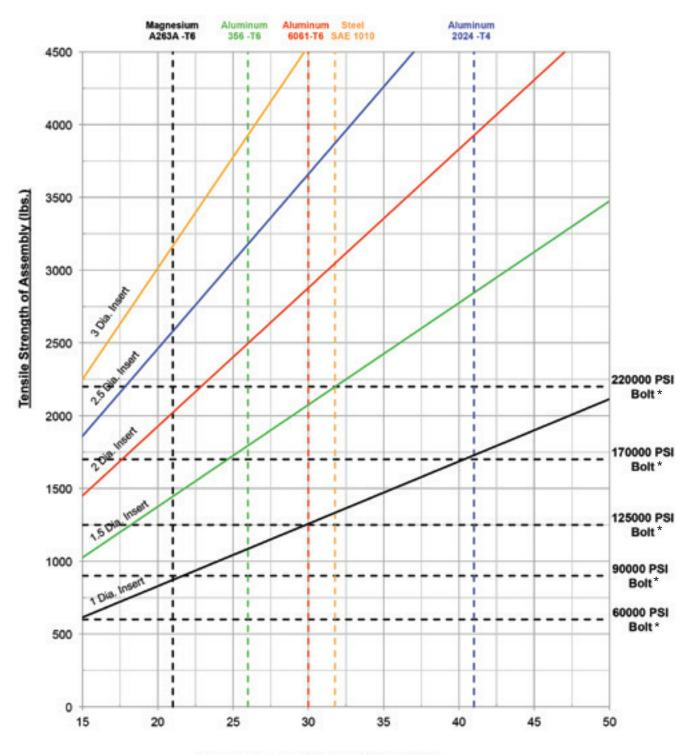
Shear Strength of Parent Material (ksi)
