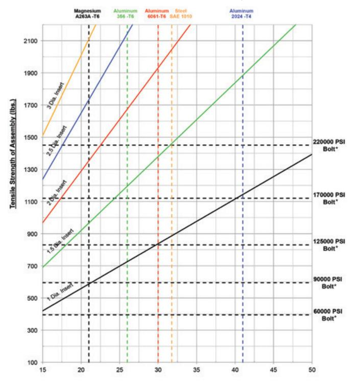
Shear Strength of Parent Material (ksi)
