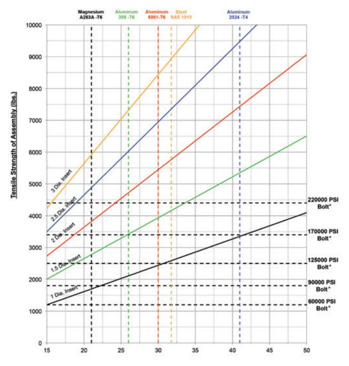
Shear Strength of Parent Material (ksi)
