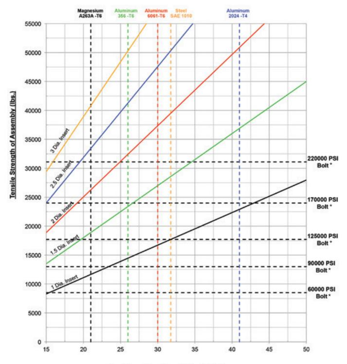
Shear Strength of Parent Material (ksi)
