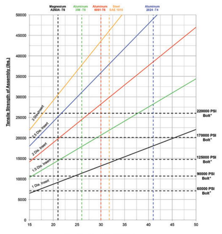
Shear Strength of Parent Material (ksi)
