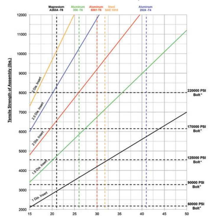
Shear Strength of Parent Material (ksi)
